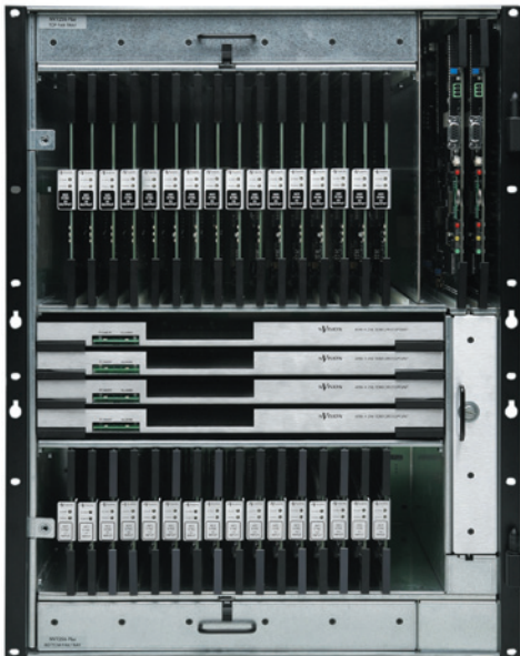
The power supplies, control module, and all the active modules are hot-swappable and plug into the front of the frame
