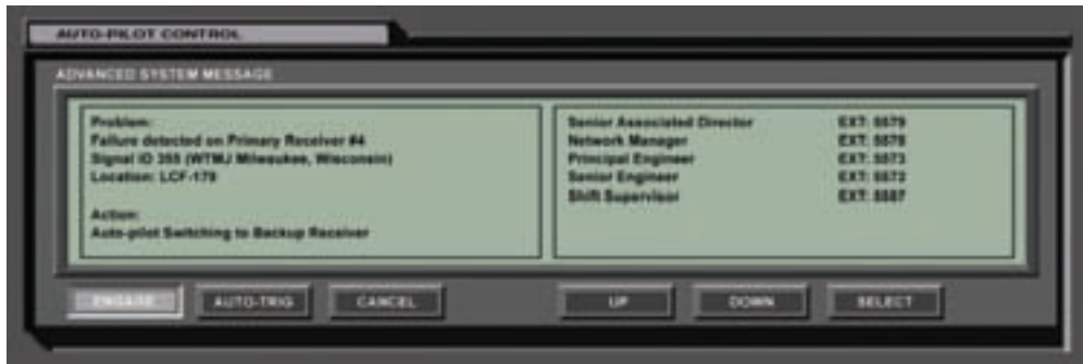
Automated response to alarms is provided by the scripted macros 'auto-pilot' function
